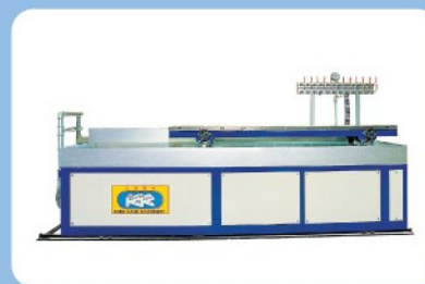
FORMING & COOLING TANK
